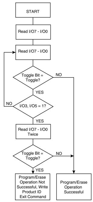
1. The system should recheck the toggle bit even if Note: I/O5 = "1" because the toggle bit may stop toggling as I/O5 changes to "1".
