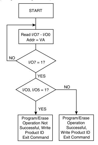
VA = Valid address for programming. During a sector erase operation, a valid address is any sector address within the sector being erased. During chip erase, a valid address is any non-protected sector address.
